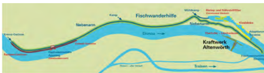
Around Altenwörth: the 12.5-kilometre-long, near-natural fish pass and the side arm of the Danube, where ecological measures have been taken.
