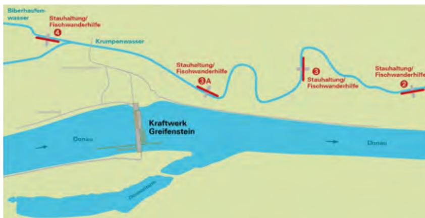
Always passable: the “Gießgang” watercourse at the Greifenstein power plant was equipped with four fish passes.
